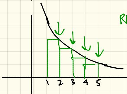
$$\begin{aligned}\text{RRAM sum} &= \Delta x \left[ f(x_2) + f(x_3) + f(x_4) \right. \\ &\quad \left. + f(x_5) \right] \\ &= 1 \left( \frac{1}{2} + \frac{1}{3} + \frac{1}{4} + \frac{1}{5} \right) \\ &\approx 1.283\end{aligned}$$
